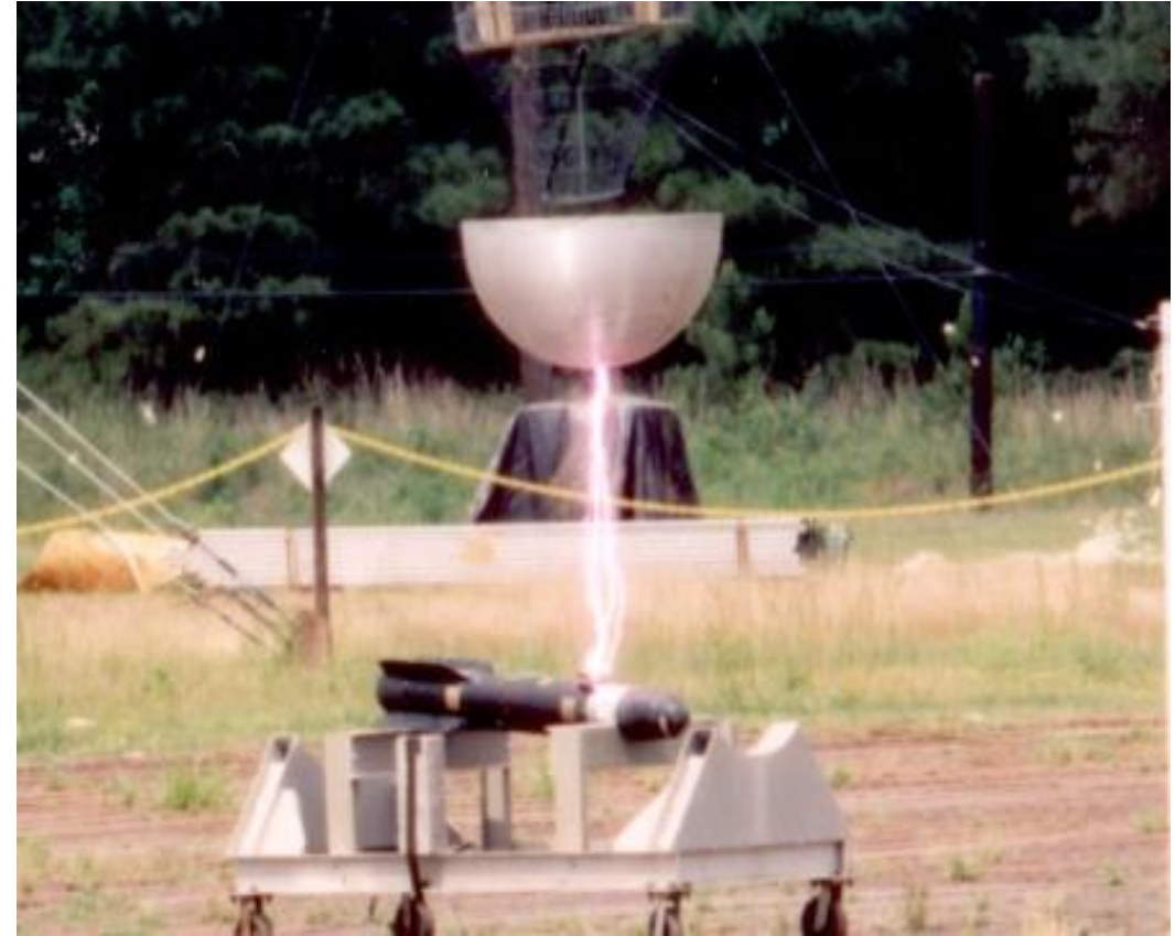
Image: Lightning Test on AGM-114 Hellfire Missile RTC, https://www.army.mil/article/163252/rtc_lightning_tests_are_on_e_of_a_kind
