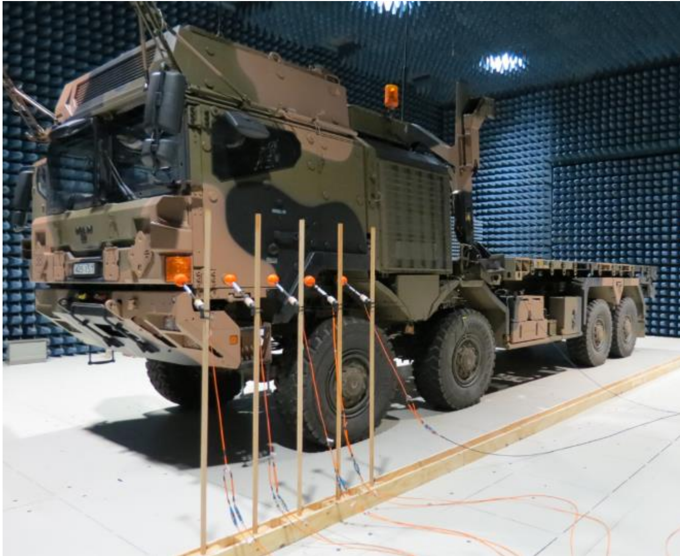
Image: ECL, RF Emissions Testing on a MAN HX-77 MHC Truck
