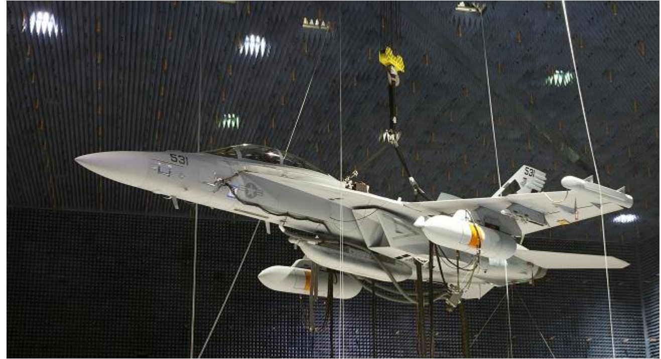
US Navy EA-18G with two NGJ-MB pods in the Patuxent River anechoic chamber. (Photo Credit: US NAVY)
