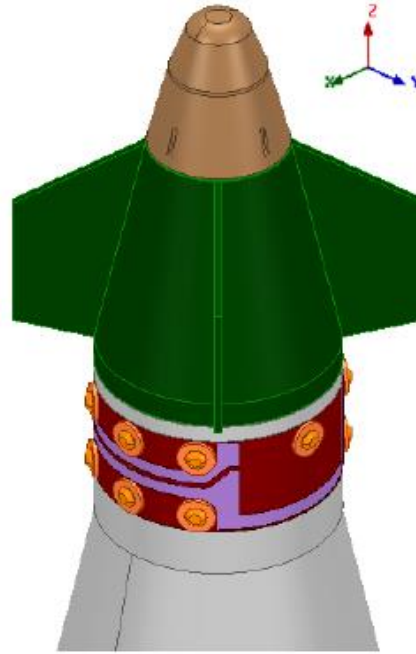
Image: A. Barton, Wraparound Antenna for S-Band Telemetry, Technical Report ARMET-TR-18051 of Jul 20
