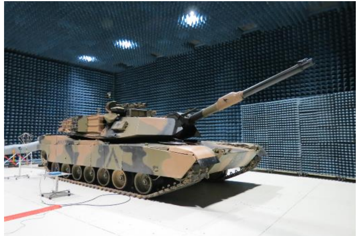
Image: M1A1 Abrams Tank in Anechoic Chamber, ECL at Monegeetta Proving Ground, VIC, Australia
